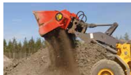
Aerating contaminated soil compost
