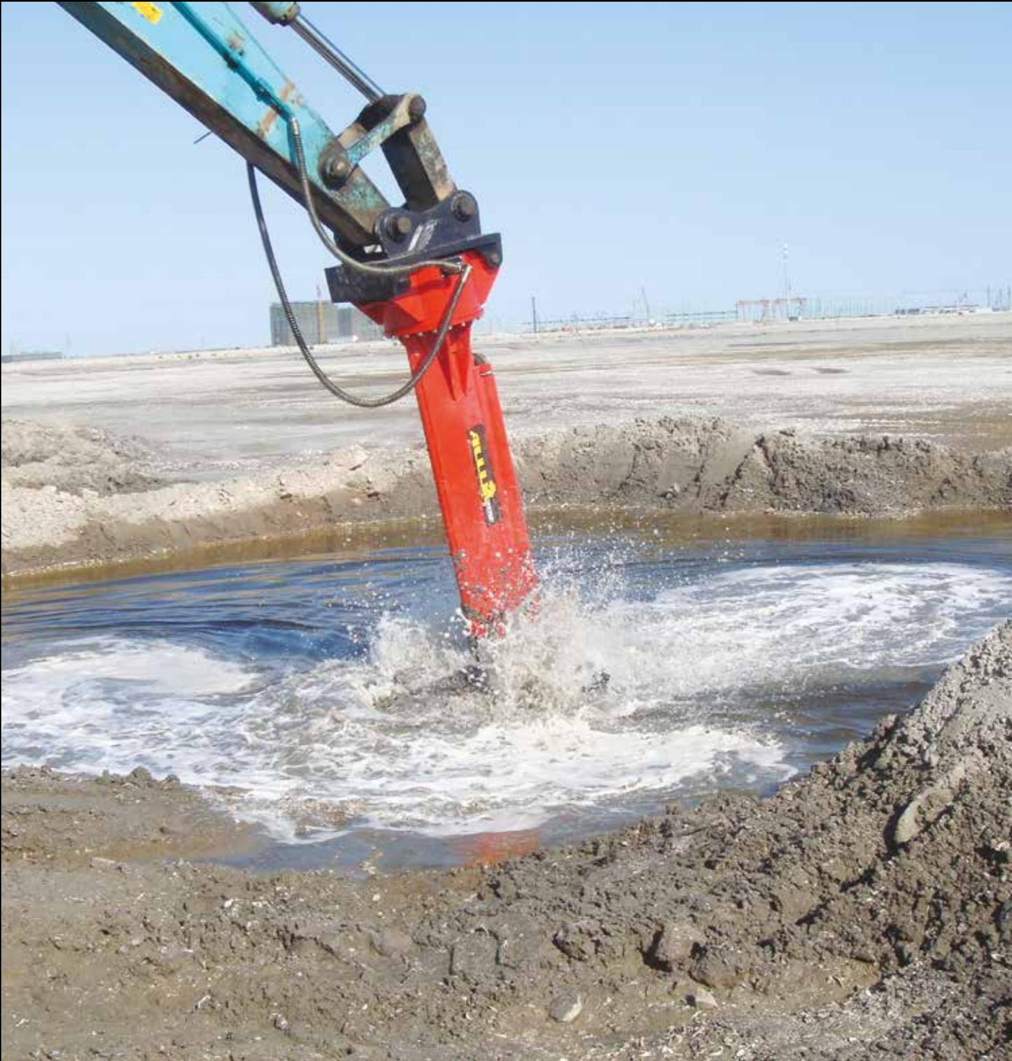
Working to a depth of 3 meters and with a weight of 2,095 kg (+400 kg fabricated mount plate), the Processor 300 HD is designed to be durable. It's made from wear-resistant steel, with a stem that's engineered to be strong, streamlined and lightweight.
