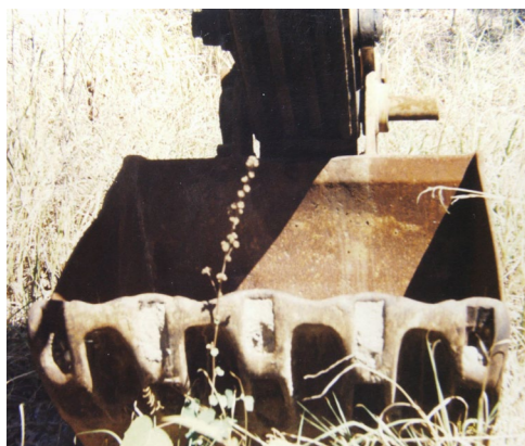
1.2m wide GP bucket with worn teeth & adaptors
