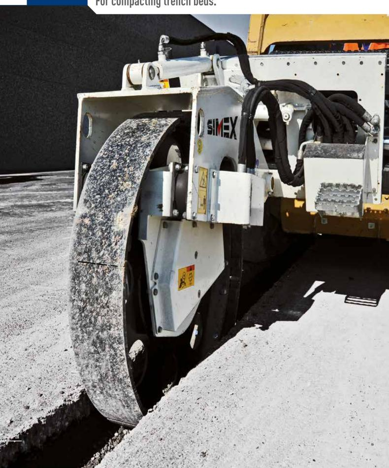
■ Designed for **compacting trench beds**, Simex CT vibrating wheel compactors guarantee a permanently firm, even and well compacted bed and ensure maximum road safety.
